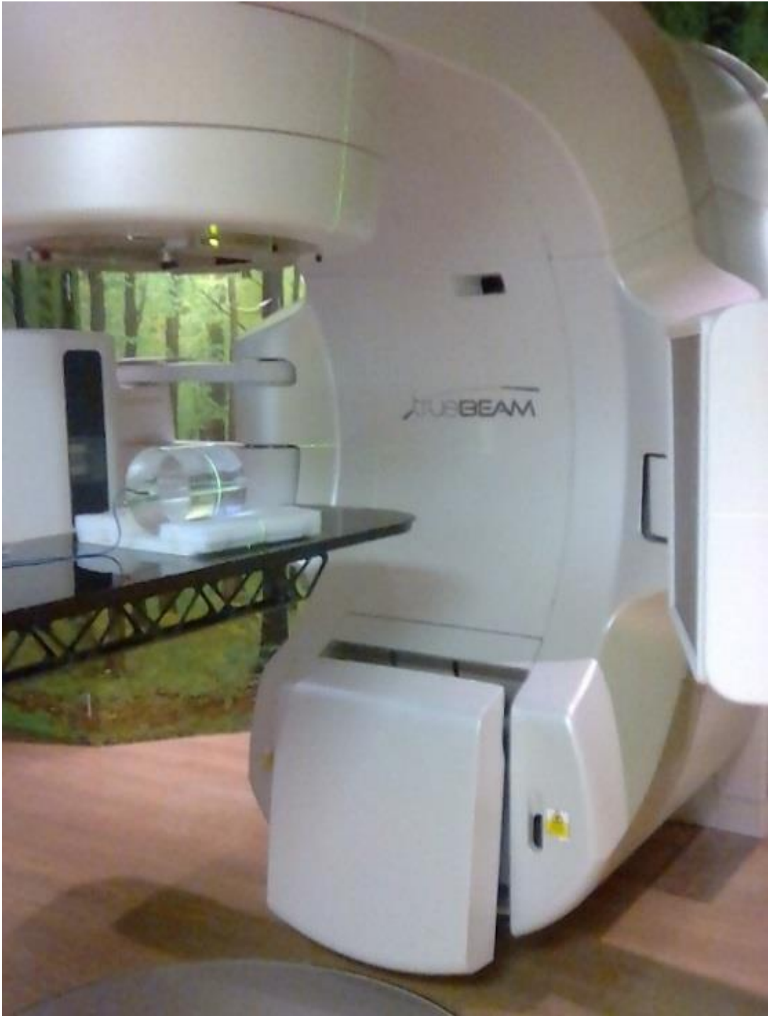
Fig. 15. Alignment of the phantom using room lasers is shown.
