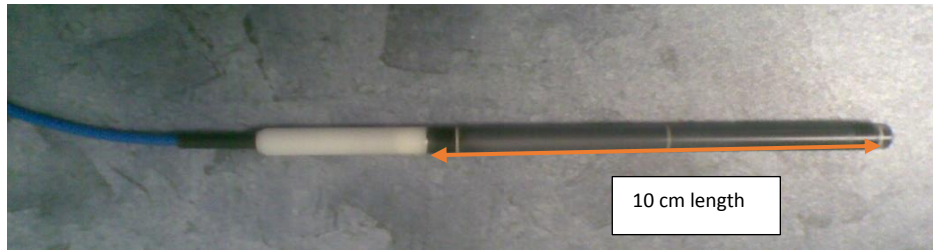
Fig. 8. The CT PTW 30009 pencil ionization chamber (PTW Freiburg, Germany) with sensitive length of 10 cm is shown. The ion chamber calibration factor used during measurements is traceable to Bureau International des Poids et Mesures (BIPM) 37 . BIPM is the international laboratory with the primary role of development and maintenance of standards.
