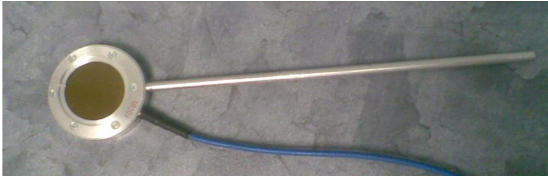
Fig. 10. The PTW TM77334 parallel plate ionization chamber (PTW Freiburg, Germany) is shown. The given calibration factor for the ion chamber was traceable to BIPM.
