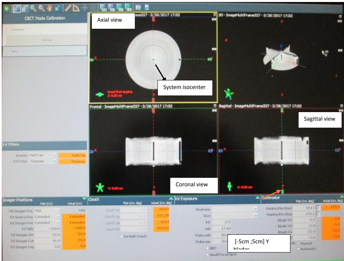
Fig. 16. CBCT image acquired for the verification of the phantom alignment is shown. On the axial view, the actual isocenter of the system is indicated by the intersection of the green and red dotted lines, and the setup isocenter is indicated by the ion chamber located at the center position of the phantom. The alignment is indicated for axial, coronal and sagittal views.
