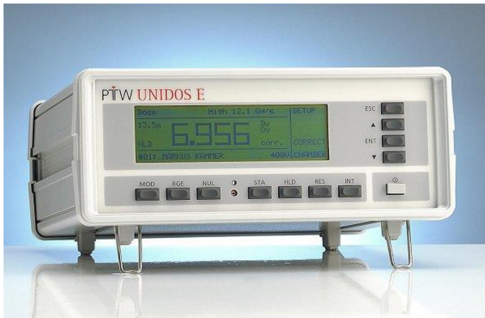
Fig. 11. The PTW 10008 Unidos E electrometer (PTW Freiburg, Germany) used for the measurement of charge during CT, CBCT dosimetry and kilovoltage dosimetry on a radiotherapy simulator and Varian OBI is shown. (image copied from ref. 39)
