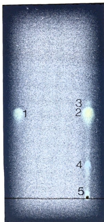
Figure 5.3 Photograph of a chromatoplate viewed at 256 nm showing PL HCl decomposition products. (1) PL HCl standard, (2) PL HCl sample exposed to 55°C, 75% RH for 2 weeks, (3) decomposition product R_f 0.48, (4) decomposition product R_f 0.17 and (5) decomposition products at R_f 0.
