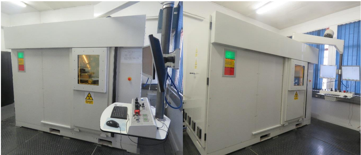
Figure 5. Nikon Metrology XTH 225/320 LC Micro-CT scanner.
