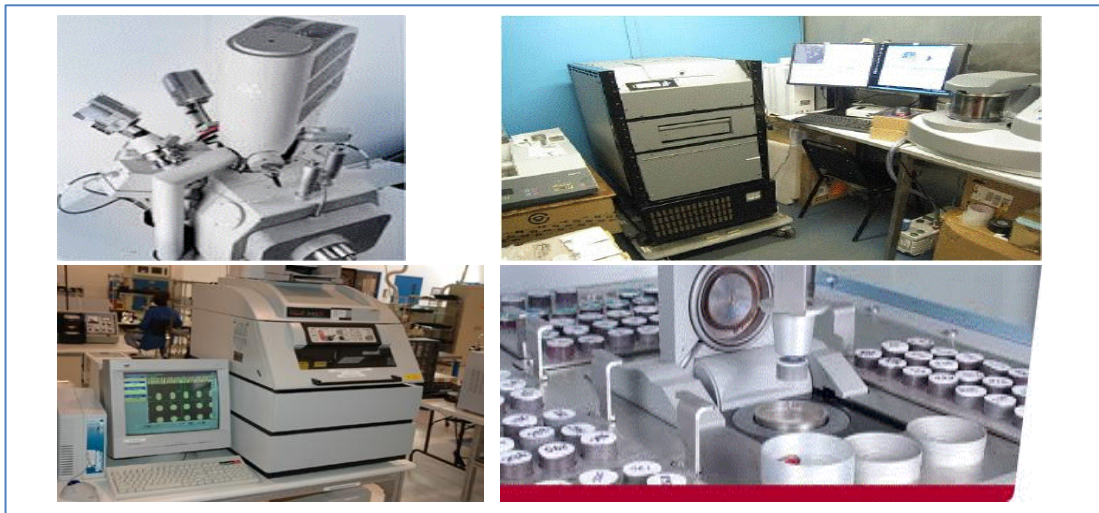
Figure 3.1: Typical XRF and QEMSCAN Set-up in Sishen and Anglo Research labs
