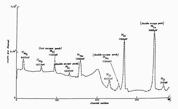
FIGURE 1. Gamma spectrum of an irradiated enamel sample 15 seconds after irradiation.
