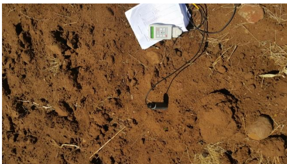
Figure 4. Field based spectroscopy for SOC content measurement: (a) Spectral measurement by ASD; (b) site localisation (Pictures captured by Dr. Elhadi Adams).
