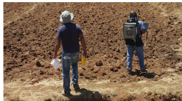
Figure 4. Field based spectroscopy for SOC content measurement: (a) Spectral measurement by ASD; (b) site localisation (Pictures captured by Dr. Elhadi Adams).
