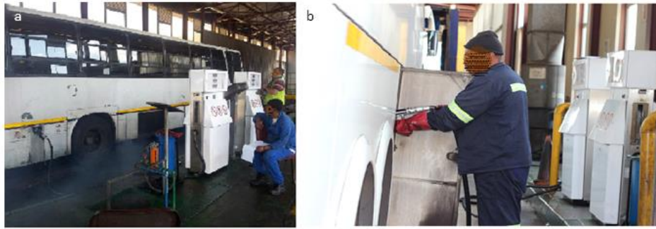
Figure 5.1: Refuelling of buses by attendants: (a) Exhaust fumes can be seen faintly near the tyre well which adds to the vapours released from refuelling. (b) Close proximity to vapours during refuelling of buses. Protective gloves are worn during refuelling, but removed while engaged in other activities as can be seen in (a).
