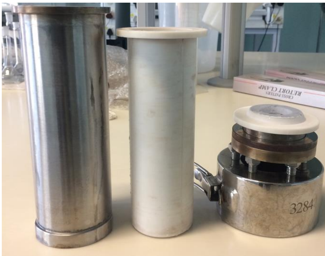
Figure 3.3: Picture of the Teflon ® -lined autoclave used for the pore-plugging hydrothermal synthesis for nanocomposite sodalite / ceramic membrane (Picture not to scale).
