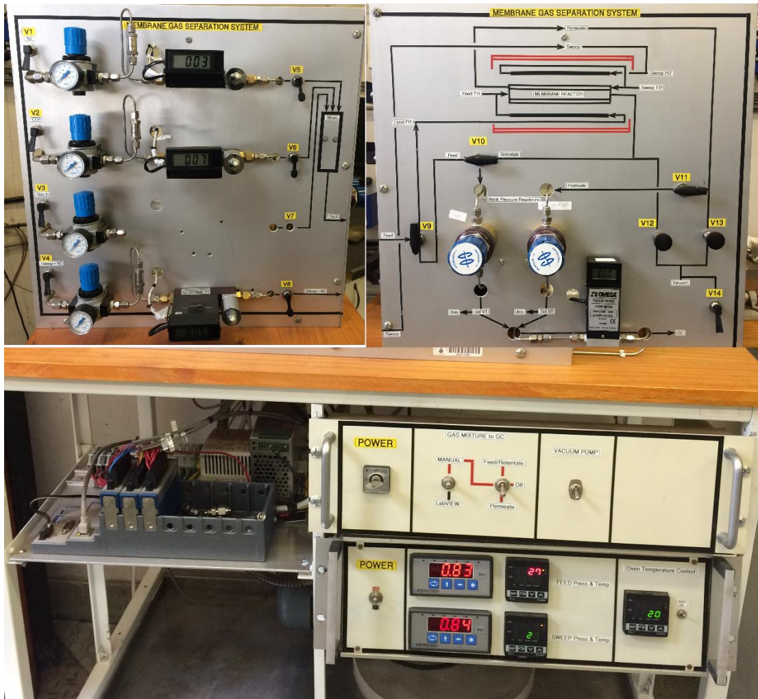
Figure 3.5: Picture of the membrane gas separation system (Picture not to scale).
