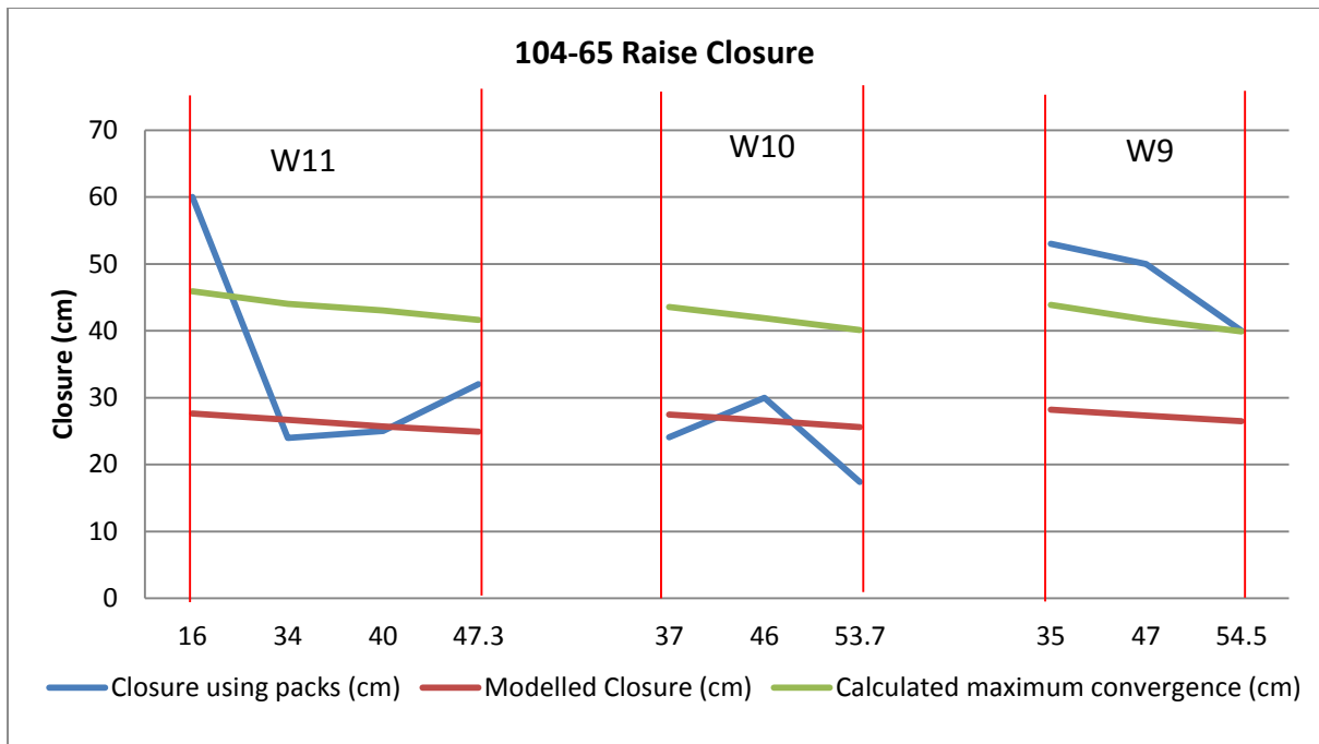
Figure 49. Closures determined at each point in 104-65 raise.
