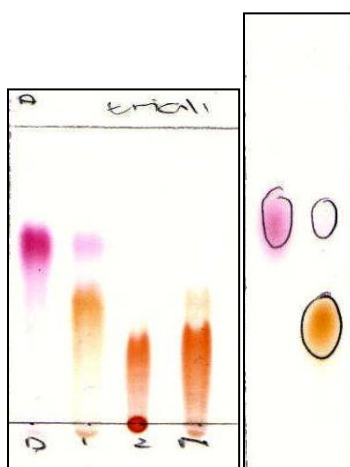
Figure 3.18 Alumina TLC plates indicating the effect of triethylamine (5% (left) and 10% (right) of the entire volume of the solvent system) on the streaking of bands observed when an EtOAc:hexane:MeCN (10:0.1:1.0) system was used.
