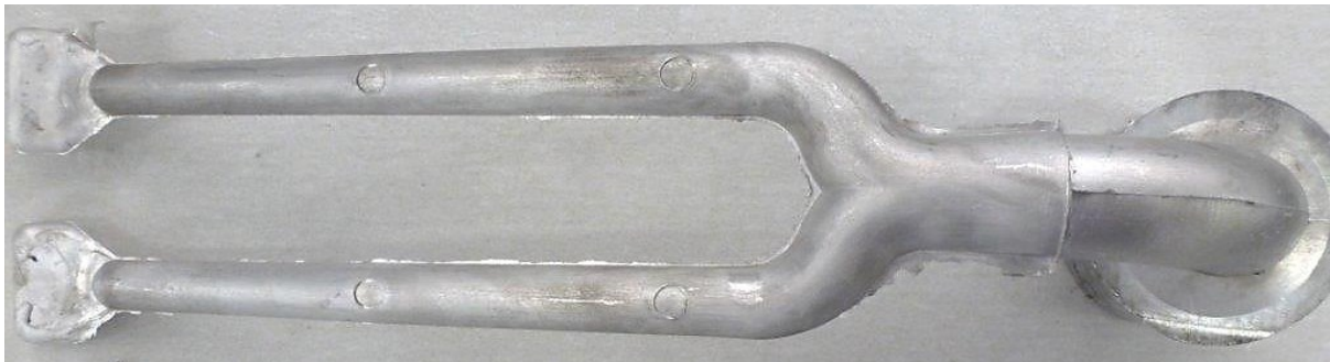
Figure 4.1. Example of the surface of the taper rod castings.
