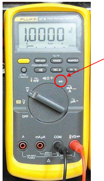
Figure 79: Diode Test Mode on Multimeter
