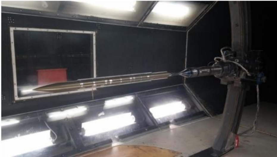
Figure 38: Model Setup in LSWT
