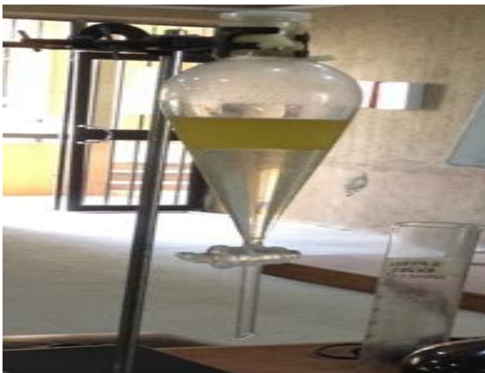
Figure F.1: Esterified oil separation into two layers
