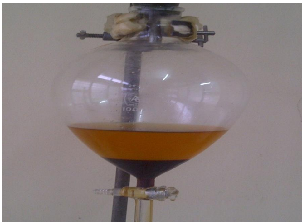
Figure F.2: Gravity settling of biodiesel, catalyst and glycerol phases
