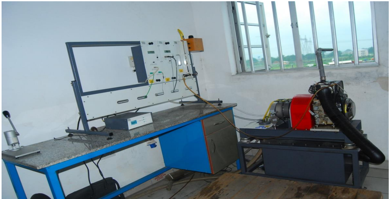
Figure 3.5: Experimental TD202 diesel test engine for performance and combustion analyses located at Petroleum Training Institute, Effurun, Nigeria
