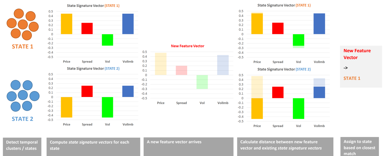
FIGURE 6.1: Illustration of online state assignment based on identified state signature vectors.
