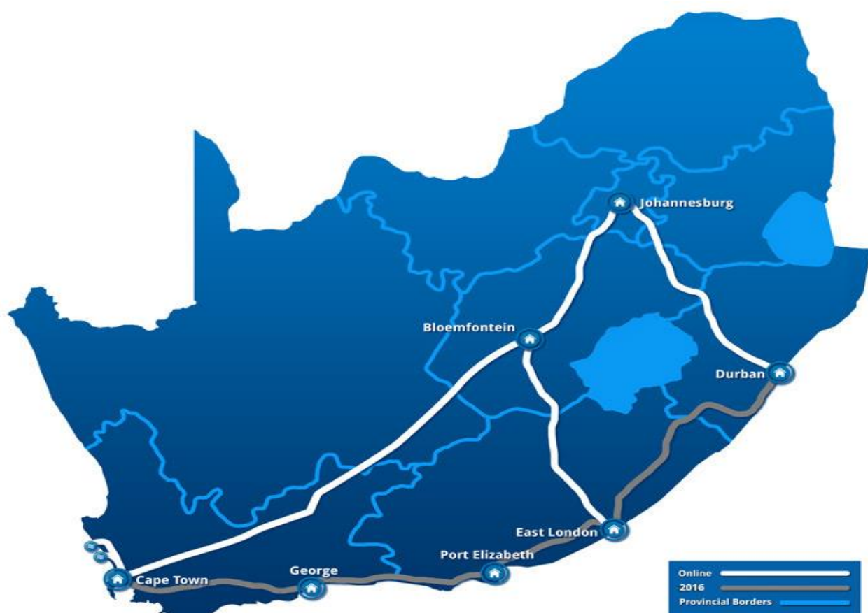
Figure 49: FibreCo fibre network across South Africa
