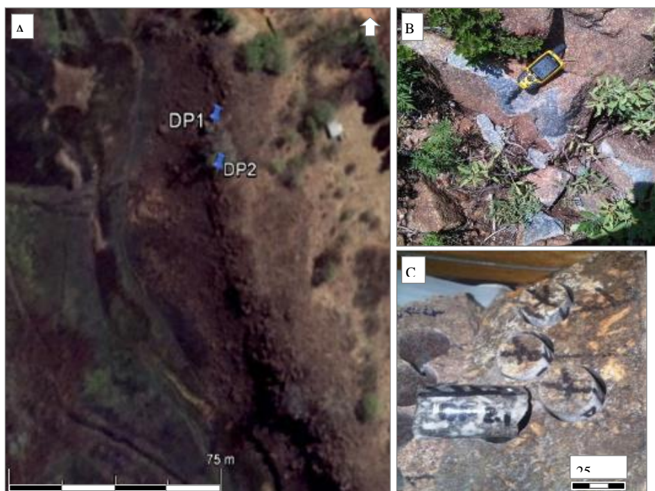
Figure 2.11 A) Site 2 along a grey syenite dyke. The whole rock sample is observed in B), and finally, the oriented core samples extracted for the physical property study in C)
