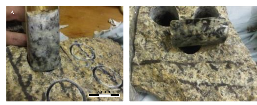
Figure 2.16 The whole rock core samples of the Pilanesberg Complex white nepheline syenite. A) Drilled core extracted from the whole oriented rock. B) The wet core sample displays a slight green colouring.
