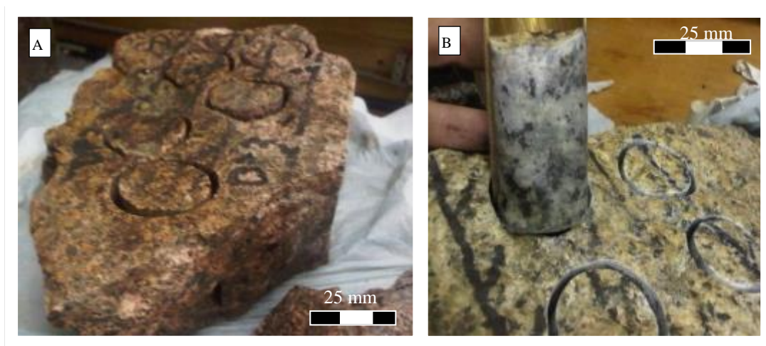
Figure 2.5 A) Red Syenite dyke whole rock sample 3 with strike lines drawn on during field measurements. The whole rock is drilled in the lab using nonmagnetic drill bits, which produce the circles. B) A copper extractor removes the white nepheline syenite core sample from the Pilanesberg Complex whole rock sample 6.
