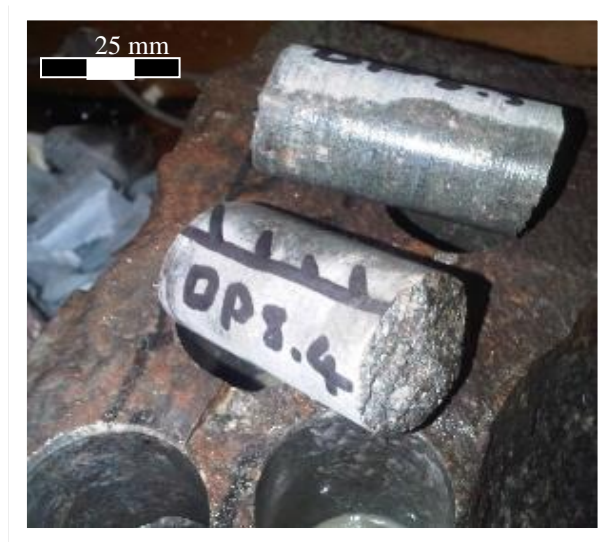
Figure 2.6 The core samples are marked with the strike and dip direction as well as sample labels. This sample is the green nepheline syenite 8.4 from the Pilanesberg Complex.
