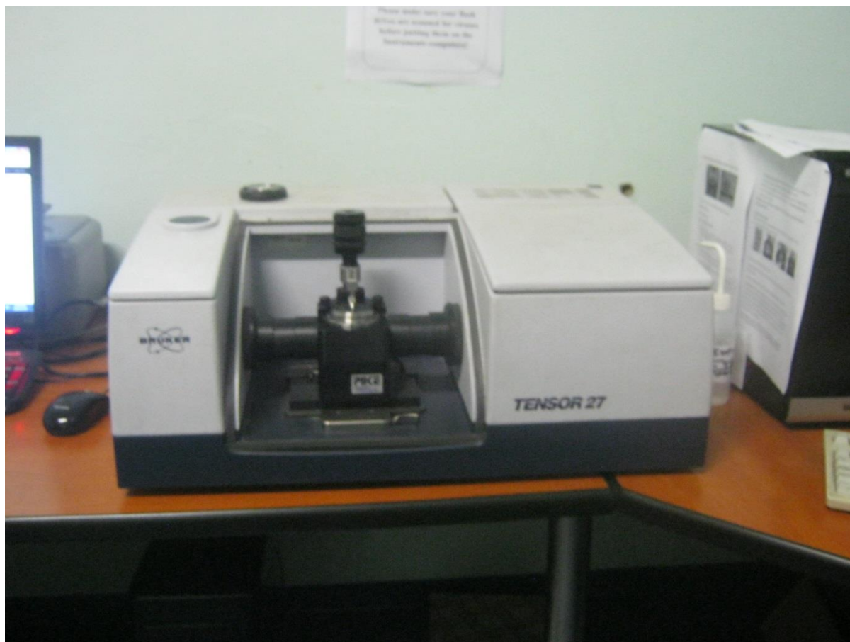
Figure 3.7: Picture of a Fourier Transform Infrared, FTIR (model Bruker Tensor 27) Spectroscopy; Bruker Germany, (Wits, School of Chemistry).
