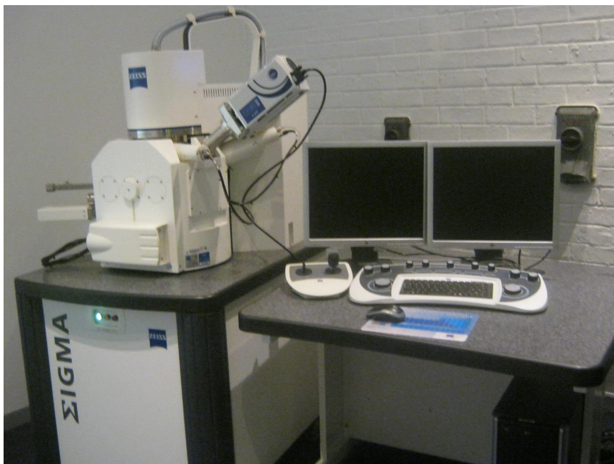
Figure 3.6: Picture of an energy dispersive spectroscopy, EDS (model Carl Zeiss Sigma), Germany (Wits, School of Chemical and Metallurgical Engineering).
