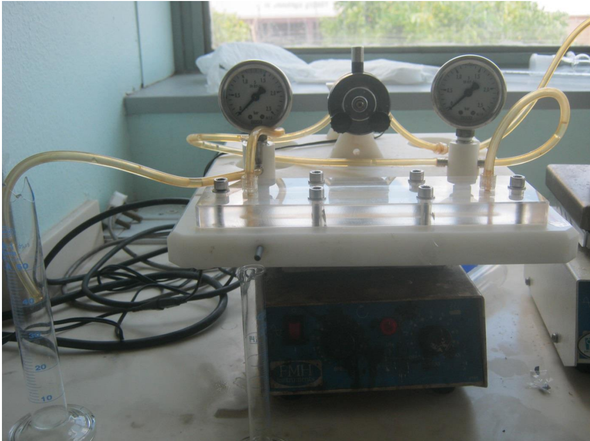
Figure 3.11: Picture of the cross flow filtration system used to separate oil-containing wastewater system.
