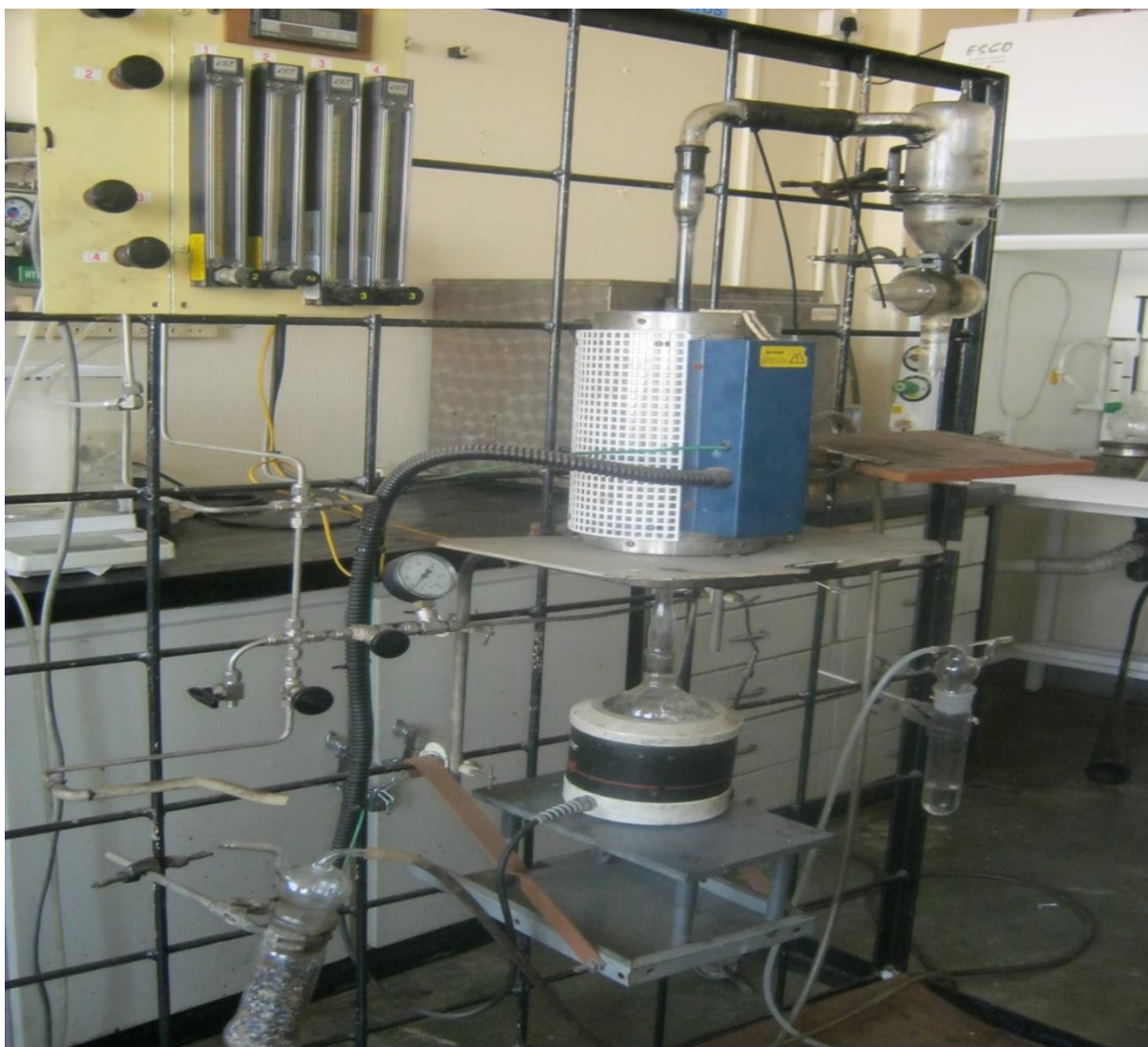
Figure 3.1: Picture of a vertical swirled fluid bed catalytic chemical vapour deposition (VSFCCVD)
