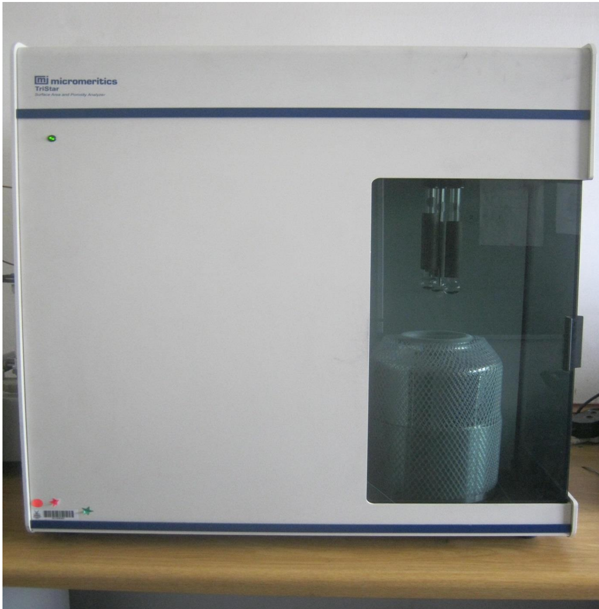
Figure 3.10: Picture of Micromeritics Tristar 3000 for the BET analysis, Micromeritics USA (Wits, School of Chemistry).
