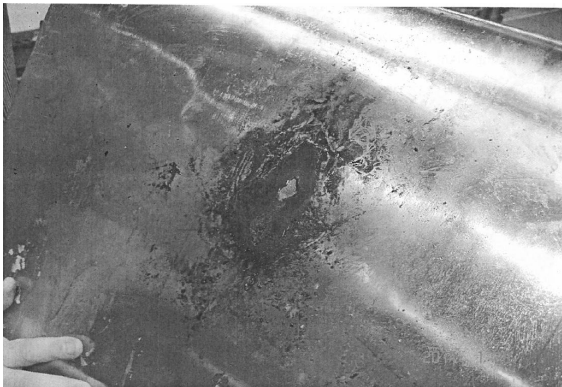
Fig. 3. Burning of first layer of LV foil winding
