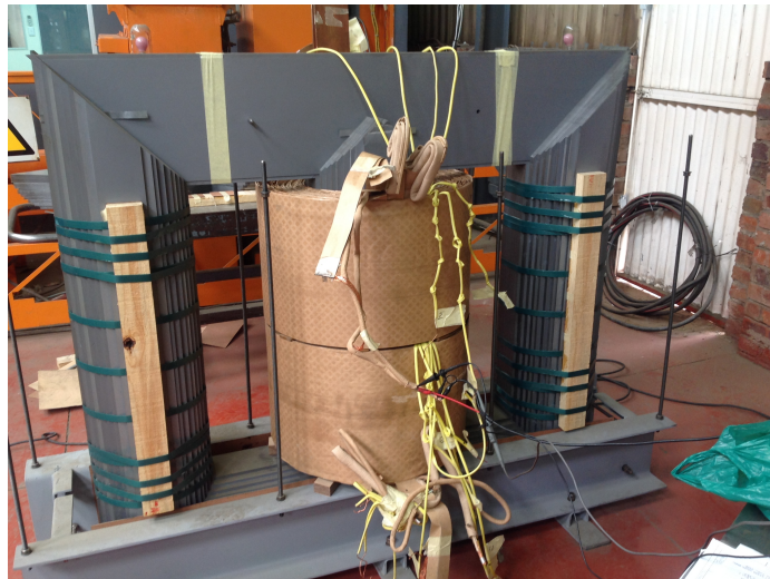
Figure 6.5: Split round winding prototype transformer.
