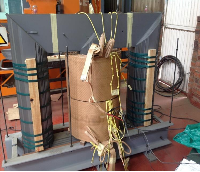
Fig. 4. Prototype transformer with measuring taps installed.
