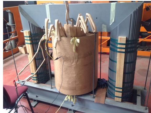
Figure 3: Prototype step-up wind turbine transformer
