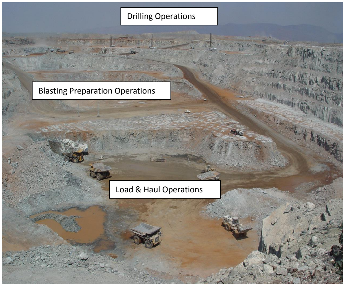
Figure 2. Activities in a typical Opencast production pit (Source: https://eureka.angloamerican.com )
