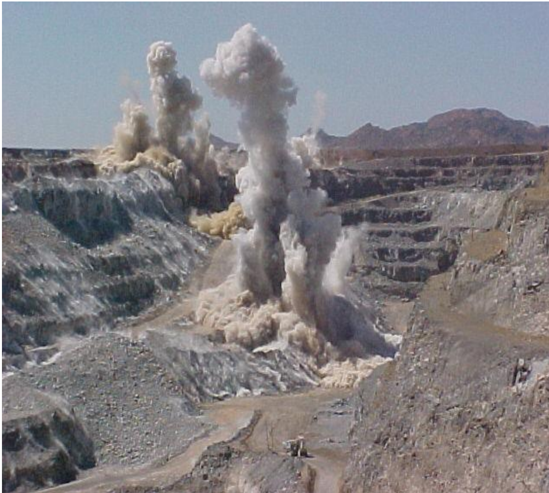
Figure 4. Rock fragmentation by means of surface blasting in an Opencast production pit (Source: https://eureka.angloamerican.com )
