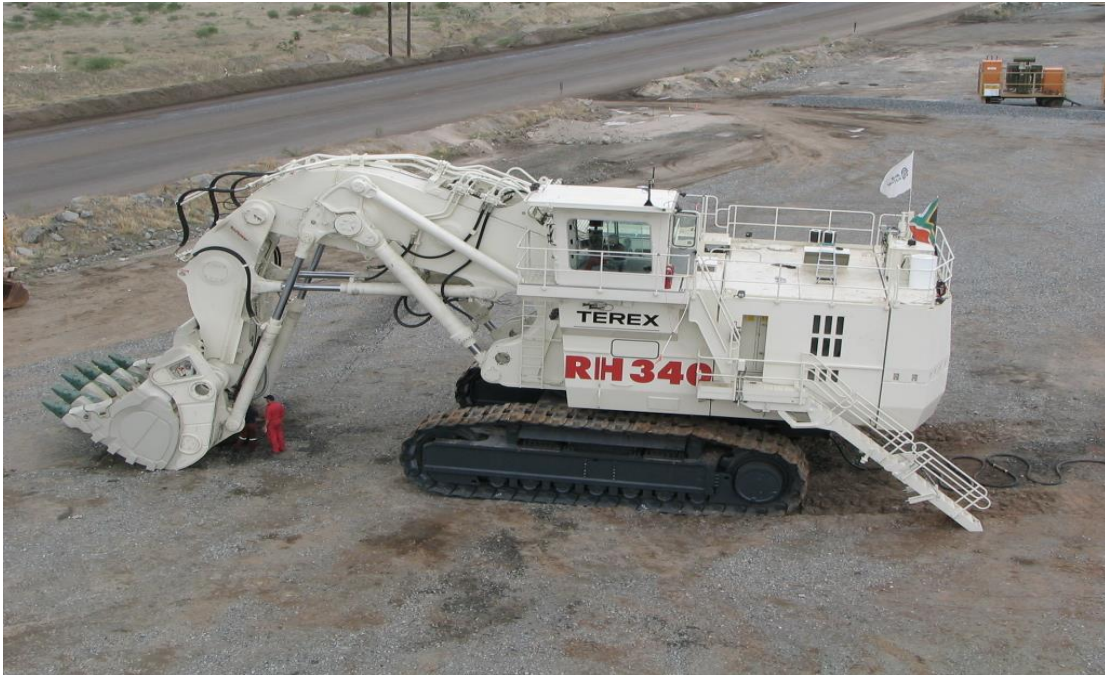
Figure 5. Hydraulic shovel used in loading dump trucks in Opencast production pit(Source: https://eureka.angloamerican.com )
