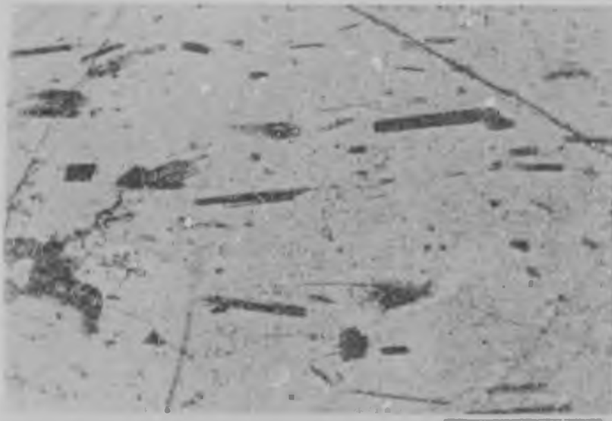
Figure 15: Rutile needles in quartz in a quartzite from the Farm Artonvilla (7 km east of Messina - see Horrocks, 1975). Scale bar is approximately 0,5 mm.
