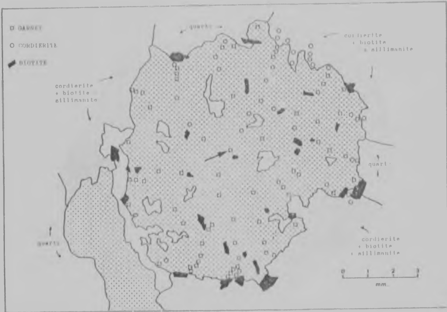
Figure 62: Schematic representation of the garnet porphyroblast from a garnet-cordierite-sillimanite gneiss shown in Figure 60 showing the locations of the electron probe microanalyses made on the garnet and adjacent minerals, including the biotite fragments. The arrowed location is the nearest to the geometrical centre of the grain - see text for discussion.
