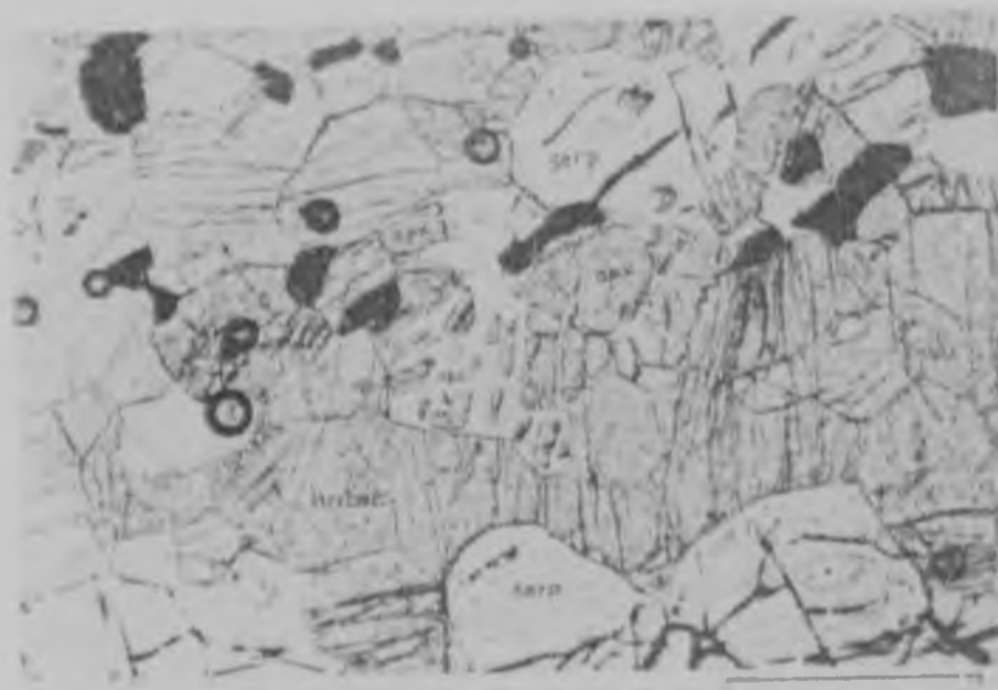
Figure 23: Serpentine (serp) replacing orthopyroxene (opx) in a serpentinite from the Farm Heuningfontein (500 m west of the main Messina -Tshipise road - see Map 1 in rear pocket). The scale bar is approximately 0,5 mm. Abundant hornblende (hnble) occurs in this rock.
