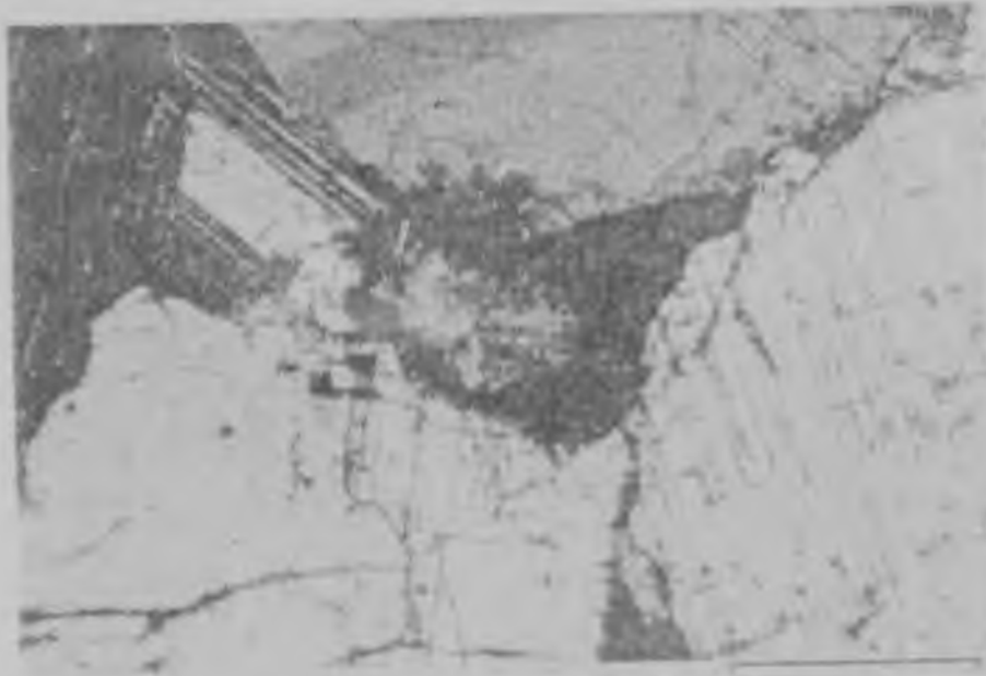
Figure 25: Interstitial altered clinopyroxene between plagioclase in an anorthositic gneiss from the Farm Shangani (4 km west of the main Messina-Tshipise road - see Map 1 in rear pocket). Scale bar is about 0,5 mm.
