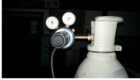
Figure 4.6: Air cylinder with pressure regulator valve
