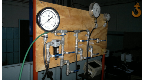
Figure 4.6: Air cylinder with pressure regulator valve
