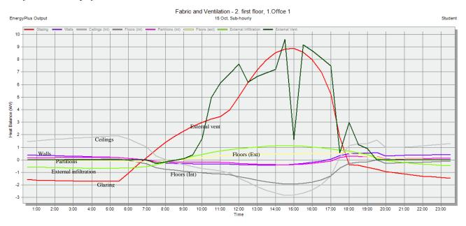
Figure 35: Example of north-western facing zone- Office 1 (red line shows glazing-peak 8.86kW). Office 2 follows similar profile
