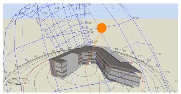
Local shading was selected from DesignBuilder templates for simplicity, permanence and for the fact that it could perform as an aesthetics feature. By modifying the existing template with bespoke model data and trying different options, the following details of the shading were specified in the model for best result over a total window area of 345m<sup>2</sup>.
