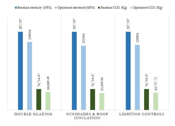
Figure 47: Comparison of results from three energy efficiency interventions
