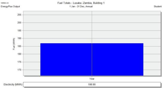
Figure 50: Simulated optimised annual electricity consumption by applying interventions 2 and 3 Tele Totals - Lusaka - Zambia, Building 1
