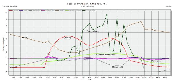
Figure 42: Optimised gains through the roof by insulation (in brown). Office zone 8 185 Fabric and Ventilation - 4. third floor, off-5
