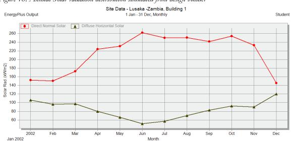
Figure 18: Annual Solar radiation distribution simulated from design builder
