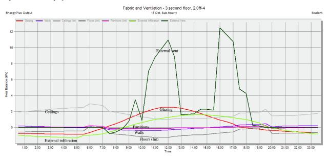
Figure 37: Example of north facing zone-Office 4 (red line shows glazing –peak 2.51kW). Offices 2, 6, 7 follow a similar profile
