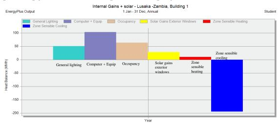
Table 19: Results after shading and roof insulation intervention.
