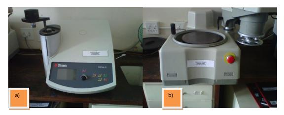
Figure 3.3: a) Struers mounting machine press, and b) Rotating grinder and polisher
