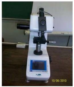
Figure 3.5: Vickers Micro hardness tester
