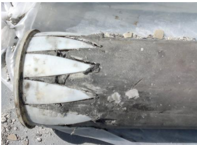
Figure 59: Core Catcher to improve recovery of wet tailings.
