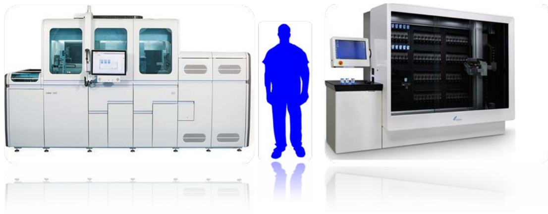
Figure 1.4 shows the current, centralized, high throughput HIV VL and TB diagnostic systems in South Africa. On the left is the Roche COBAS® 8800 VL testing platform and on the right, the GeneXpert® Infinity-80 system for TB diagnosis and RIF susceptibility testing.
