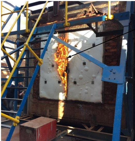
Figure 11: Flame on unexposed face of test specimen during test conducted by Firelab.
