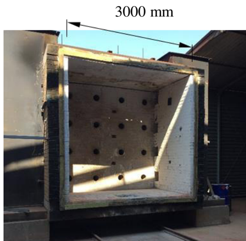
Figure 7: Firelab's vertical furnace
