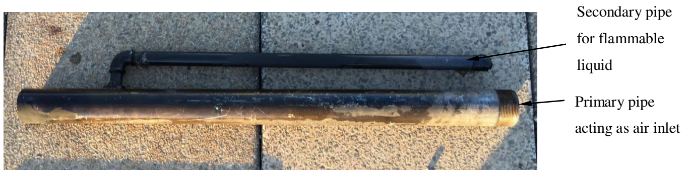
Figure 20: Burner used for preliminary flammable liquid tests
