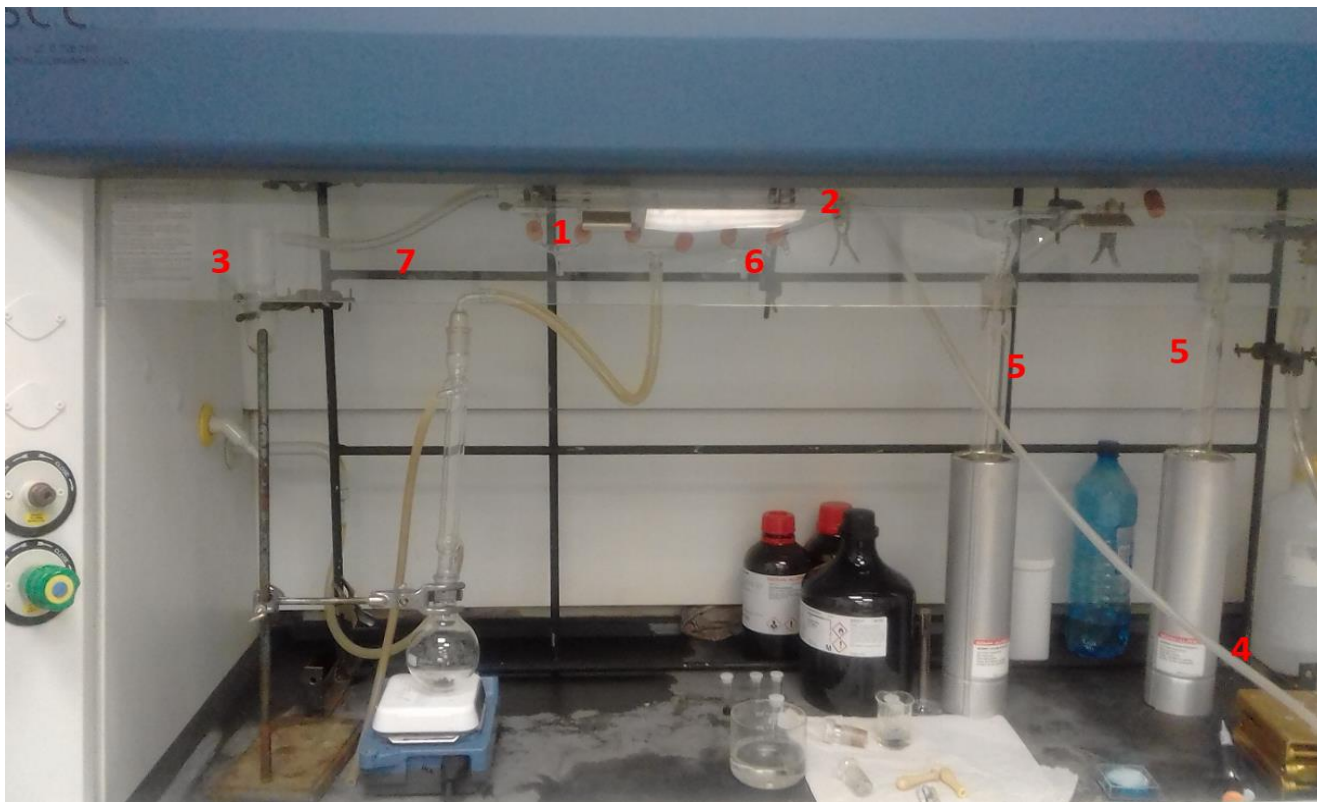
Figure 3-4 Experimental set up in the fume hood showing the complete connections for the Schlenk line
