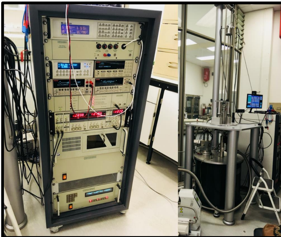
Figure 3-11 Experimental facilities showing the cryogenic high field measurement system
