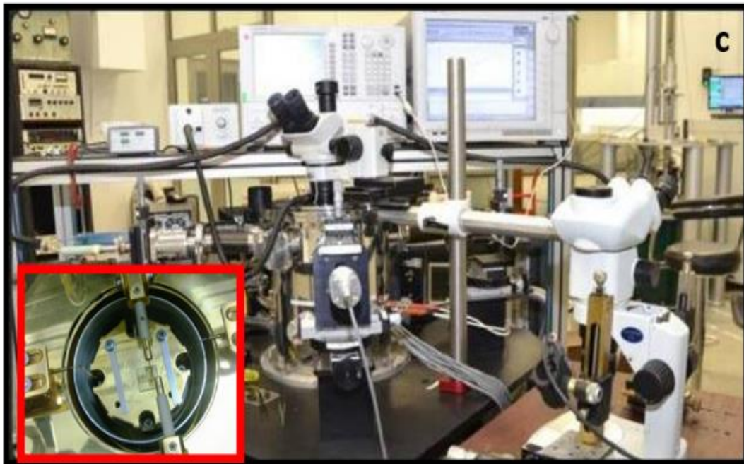
Figure 3-13 Janis micro manipulated semiconductor analyser probe station
