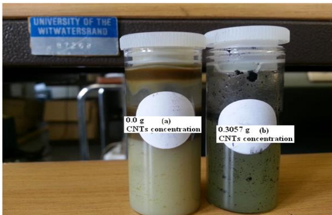
Figure 4.17: (a) initial solution of oil waste-water and (b) oily waste water containing 0.3 g of raw MWCNTS for pre-treatment by flocculation.
