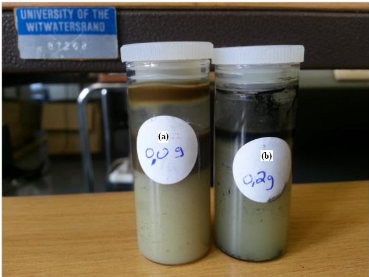
Figure 3.3: Illustration of (a) the initial solution of oily wastewater and (b) oily wastewater emulsion containing 0.2 grams of raw MWCNTs for pre-treatment by flocculation.
