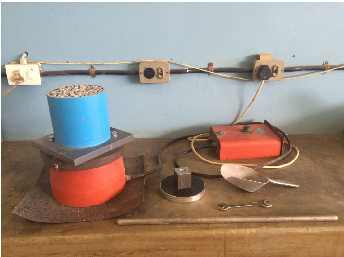
Figure 4.7: Vibration setup showing mould with specimen on vibrating table, 2 kPa circular steel surcharge, rod used to flatten surface, scoop and spanner
