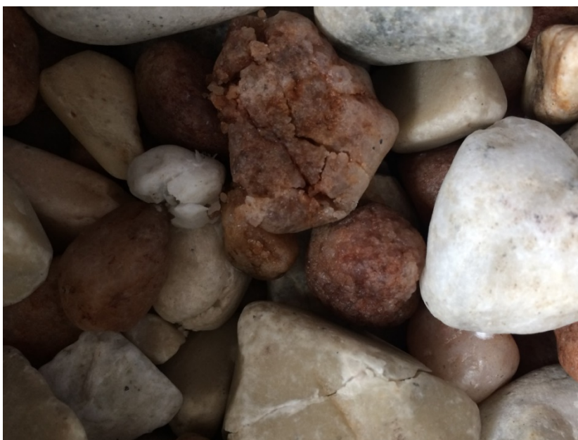
Figure 4.21: Observed pebble crushing following punch testing
