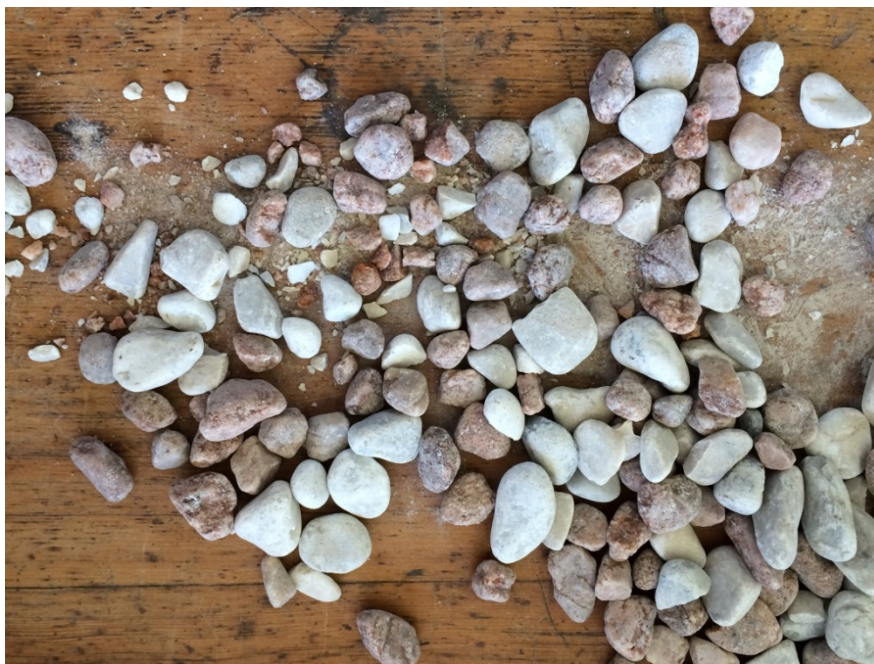
Figure 4.6: Evidence of pebble crushing during Proctor compaction
