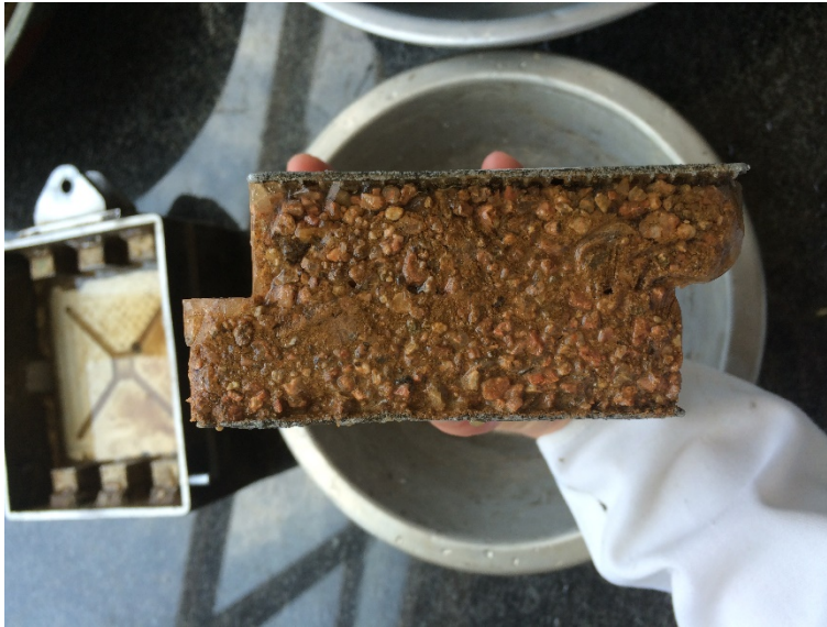
Figure 7.8: Typical frozen specimen showing sheared halves (Specimen No. S1G-F25-D-150-25_75-1)
