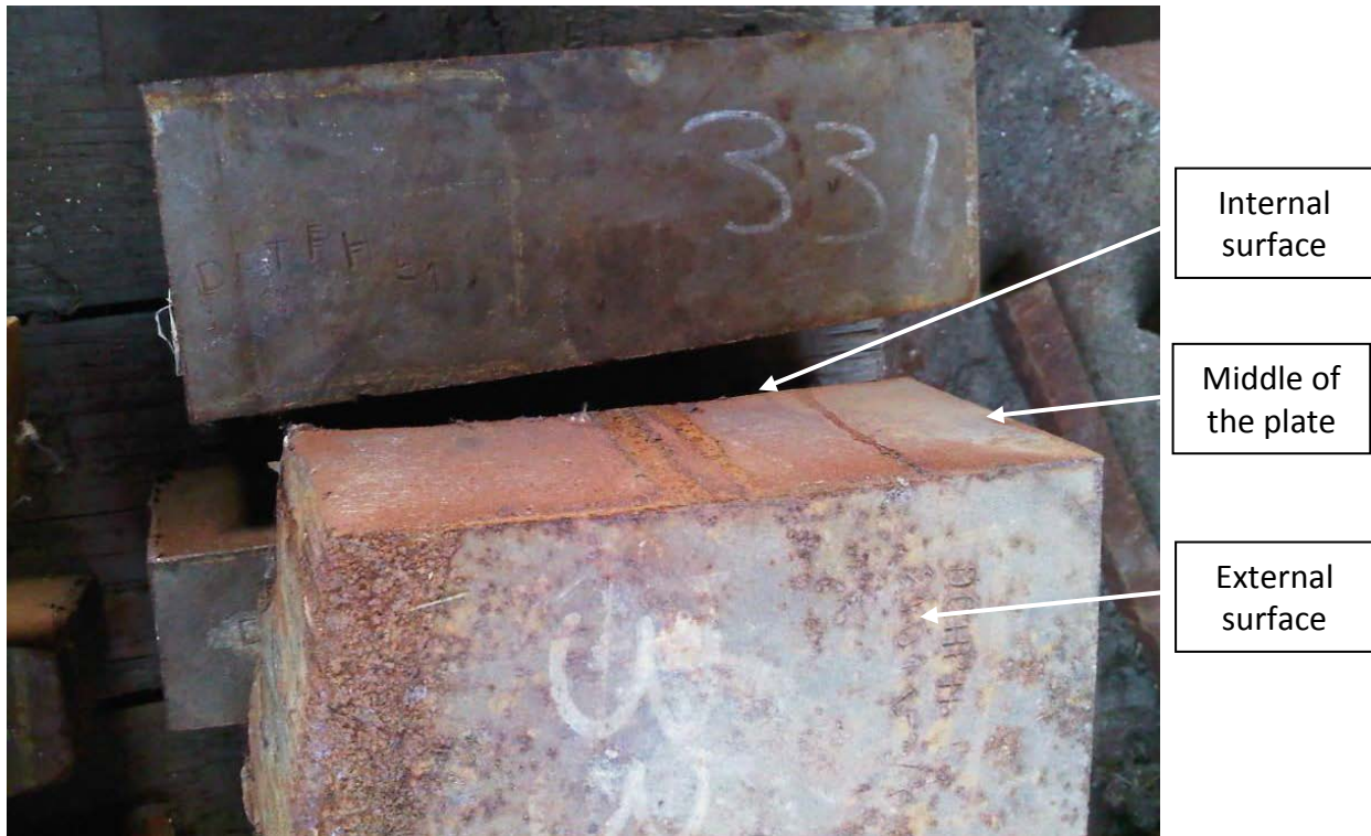
Figure 3.3: Representative photograph showing samples cut from the top dome.
