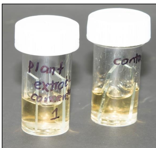
Figure 3.1: Disposable bijou bottles with sterile slides at 90°
