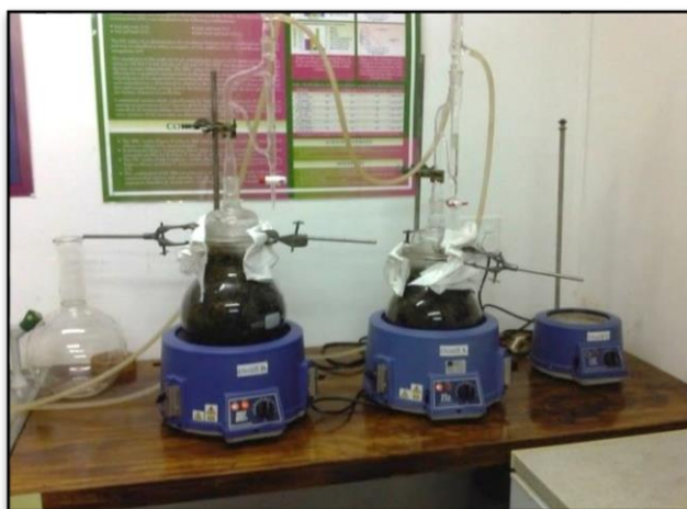
Figure 2.2: Hydro-distillation of essential oil using a Clevenger-type apparatus.
