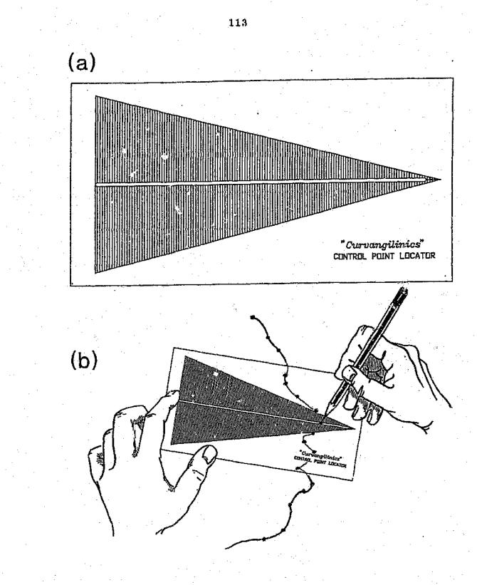
FIGURE 19 - The Control Point Locator (CPL).
