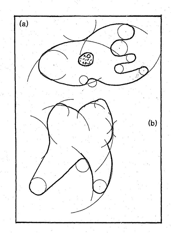
FIGURE 15 - Simplifying compound curves with simple arcs.
