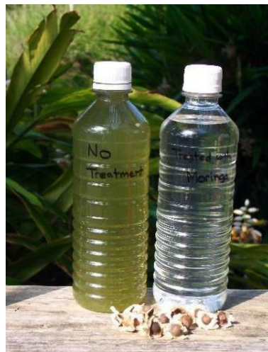
Figure 5: Moringa oleifera seeds used for water purification (Shah, 2012)
