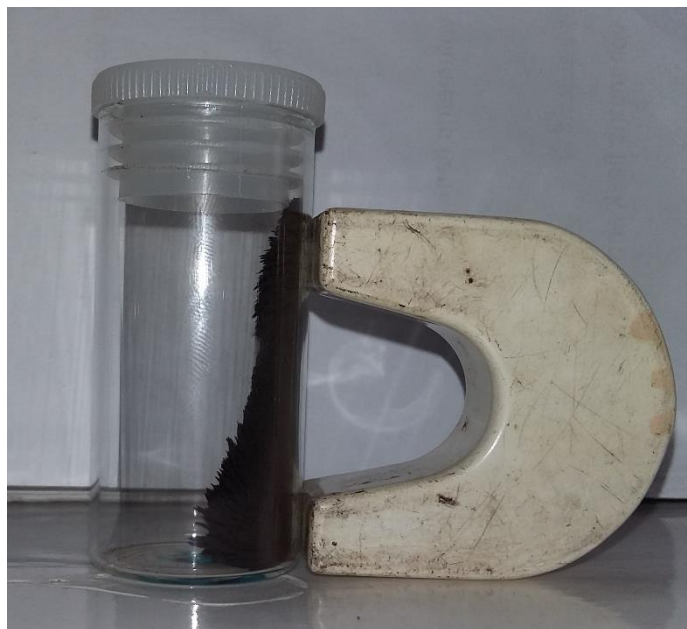
Figure 8: The response of the \text{Fe}_3\text{O}_4 due to a magnetic field.
