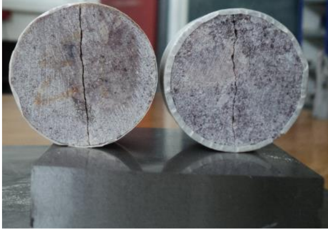
Appendix 2.1.1 Brazilian tensile test specimen after failure
