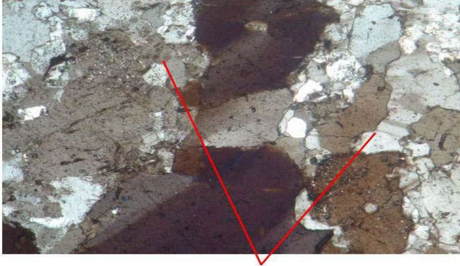
Fine-grained quartz on either side of coarse-grained quartz
