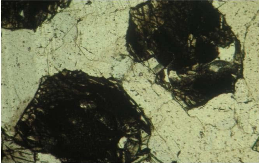
Isolated semi-rounded olivine grains with the cores partially replaced by magnetite
