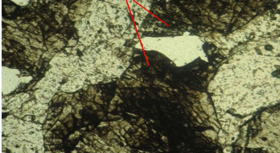
Figure 4.18 PPL photograph of a cluster of olivine grains in Troctolite2 (field of view 2 mm).
