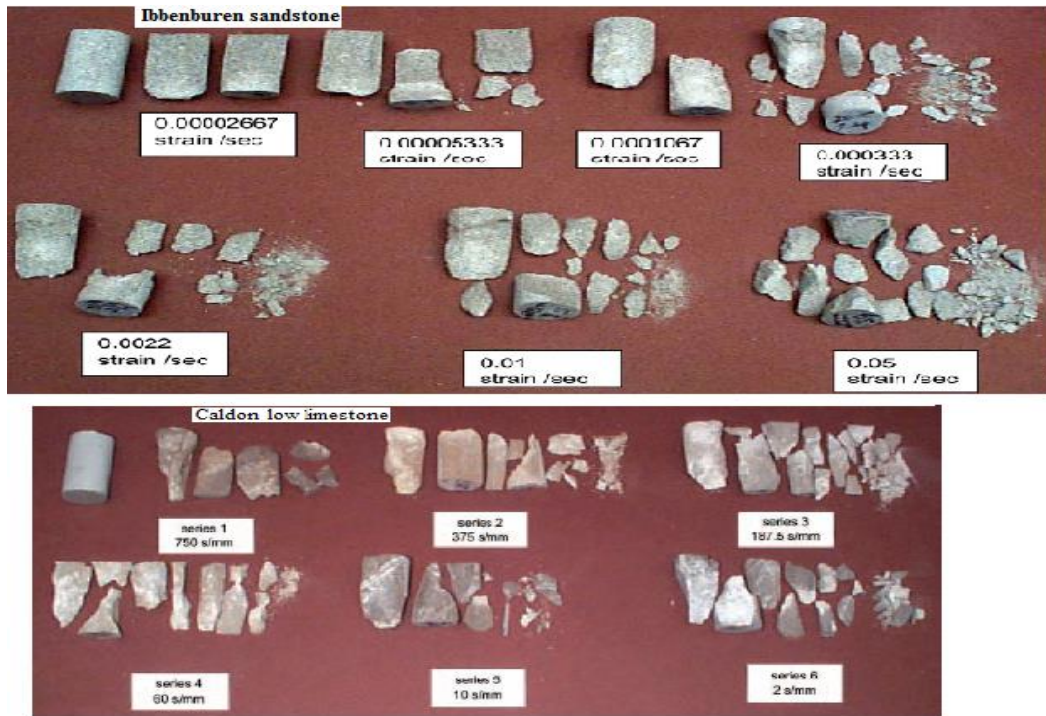
Figure 2.34 Photograph of the pre- and post-test sample core debris from the Ibbenburen Sandstone and Caldron low Limestone, showing changes in fragments size with strain rate (Whittles et al., 2006).
