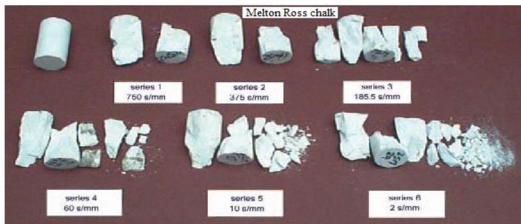
Figure 2.35 Photographs of the pre- and post-test sample core debris from the Melton Ross chalk, showing changes in fragments size with strain rate (Whittles et al., 2006).
