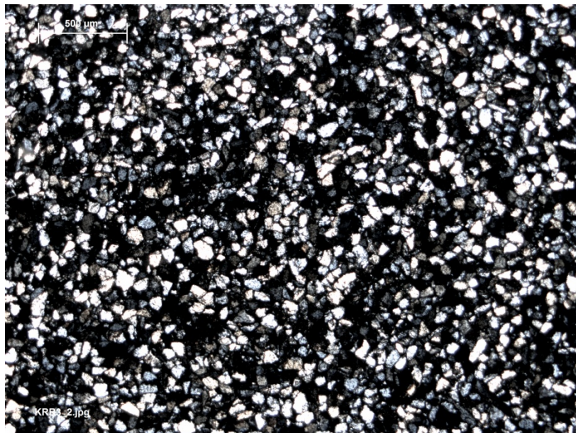
Figure B8: Thin section of FA VIII. KRR-3 is very fine-grained and quartz rich. Cross-polarized light, scale bar = 500 \mu\text{m} .
