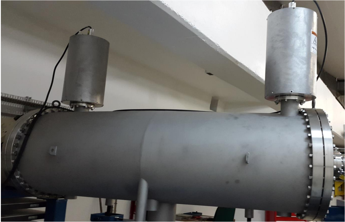
Figure 3.16: Cylindrical ESA on the higher energy system of iThemba LABS.
