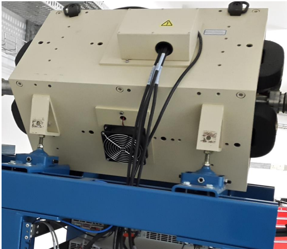
Figure 3.17: Photograph of one of the MQD of iThemba LABS.
