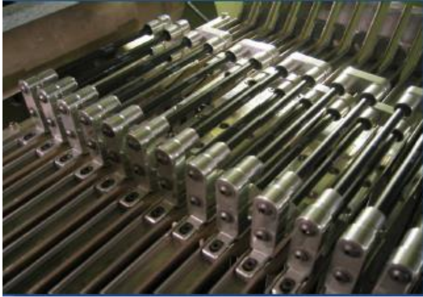
Figure 3.12: Resistors inside the tank of 6 MV Tandem accelerator at iThemba LABS.
