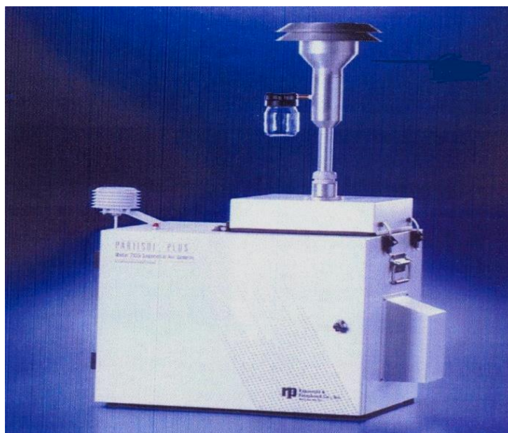
Figure 6.2: Partisol-plus sampler (Rupprecht & Patashnick, 2012).
