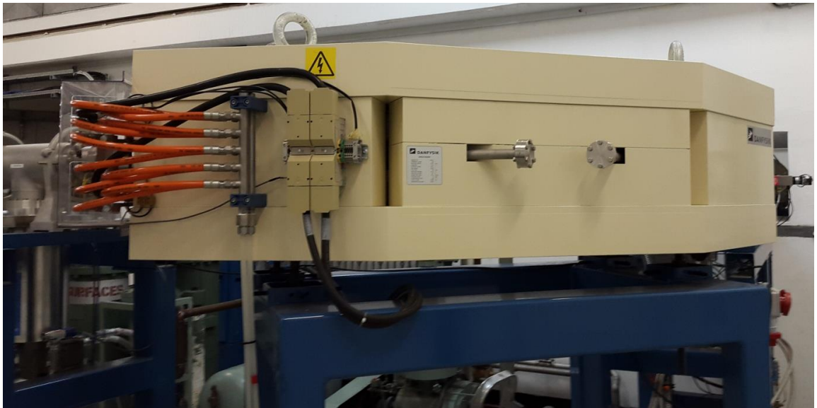
Figure 3.15: HE AMS 90^\circ analyzing magnet of the iThemba LABS
