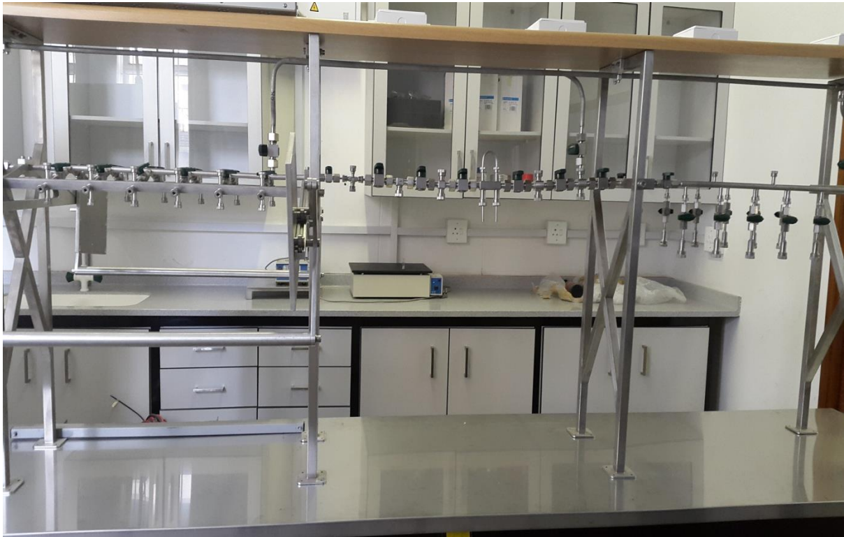
Figure 5.1: The graphitization line for sample preparation at iThemba LABS.
