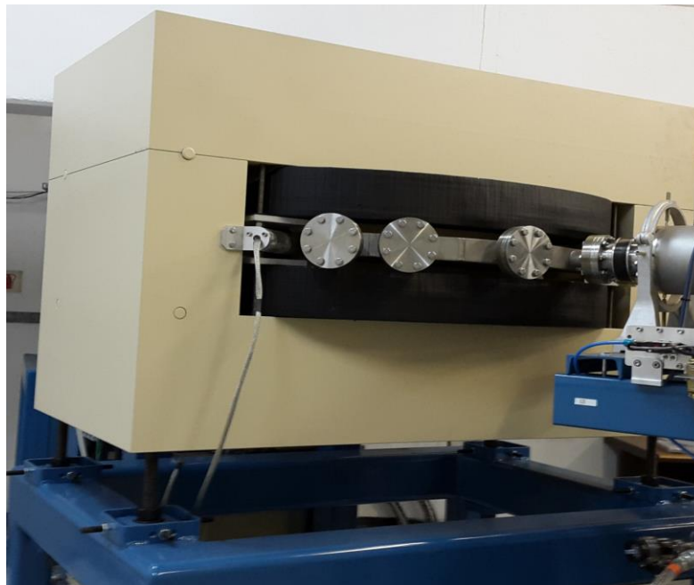
Figure 3.18: Photograph of AMS switching magnet of iThemba LABS.
