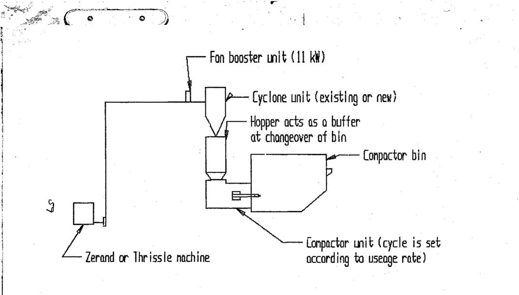
Fig. 7.5 Compactor used on Zerand and Thrissle nachines
