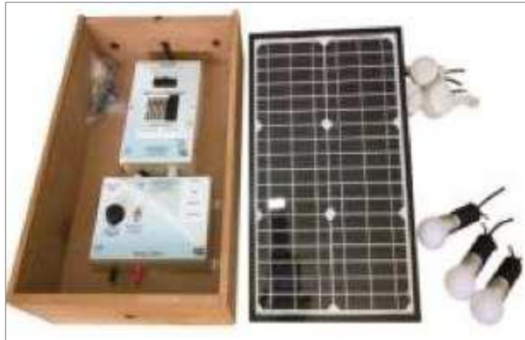
Figure 2.1: Direct current multigrid system (Source: Keller, 2012)
