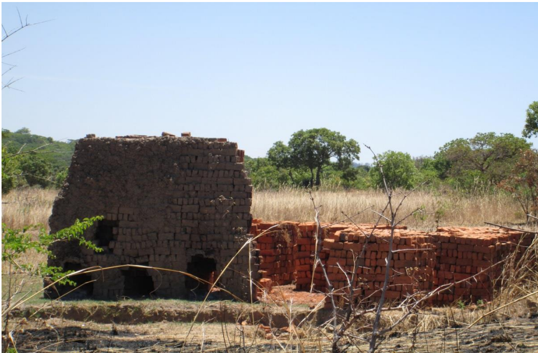
Brick kiln in a field ready for firing. In the background stacks of bricks fired and ready for selling.
