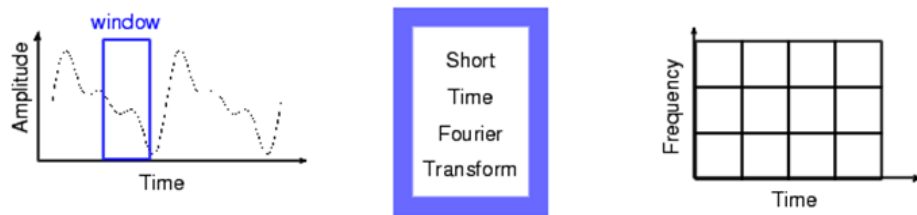
Figure 5.1 Computation of Fourier analysis using windows of the same size (Misiti et al., 1997).
