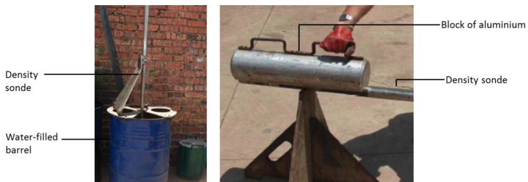
Figure 2.11 Calibration using a water-filled jig (left) and a block of aluminium (right) (modified from Chatfield, 2008).
