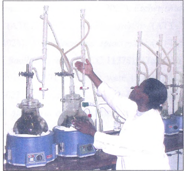
Figure 6: Hydrodistillation of plant material using the Clevenger apparatus.
