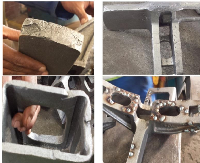
Figure 6-15: Castings after dress after Weld
