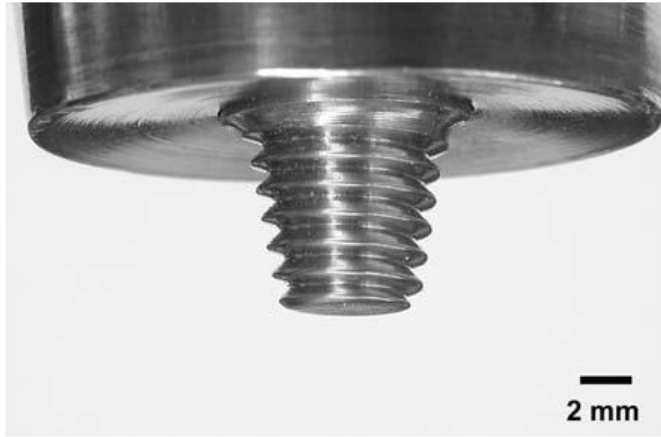
Image 3.5: Truncated cone pin and convex shoulder friction stir welding tool.
