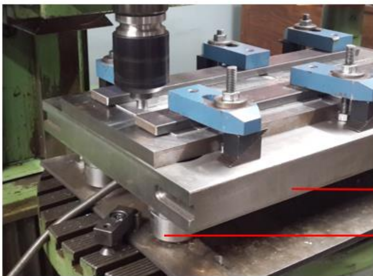
Image 12.9: Placement of the sensors beneath the backing plate
