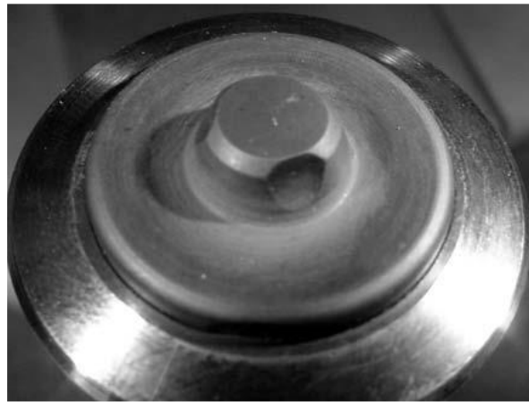
Image 3.10: Example of a threadless pin tool. Polycrystalline cubic boron nitride pin tool with three flats at pin tip.
