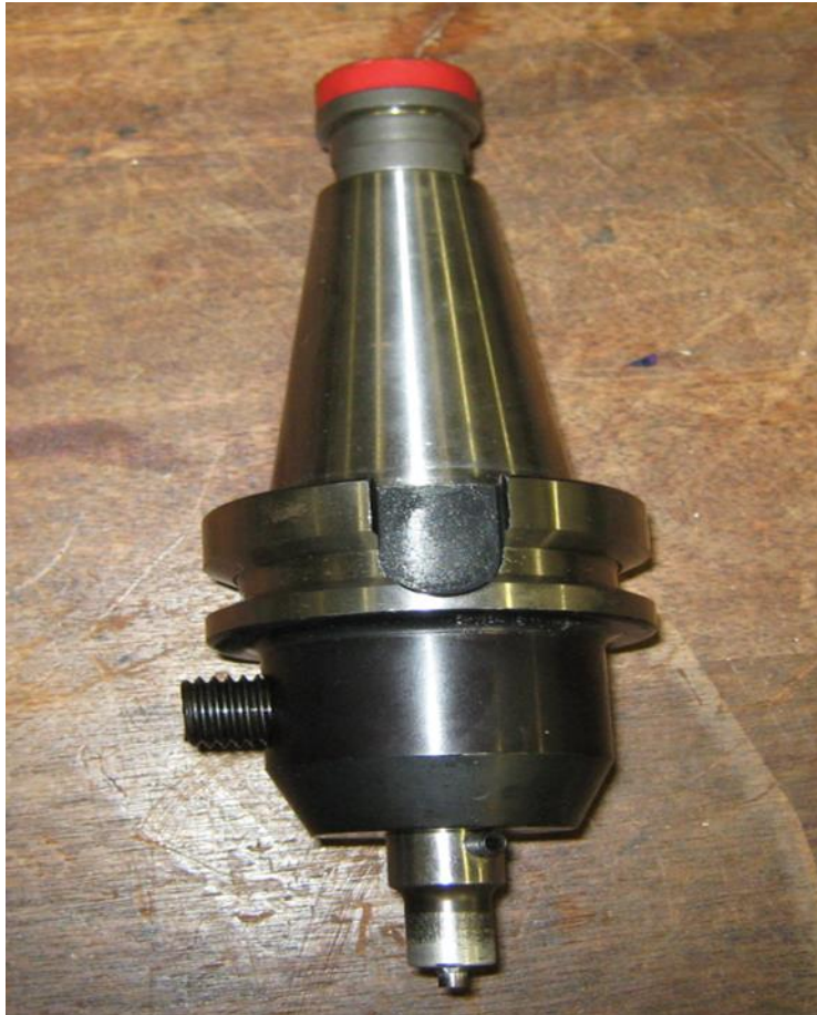
Image 12.5: The Friction Stir Welding Innovative Tool with Pin
