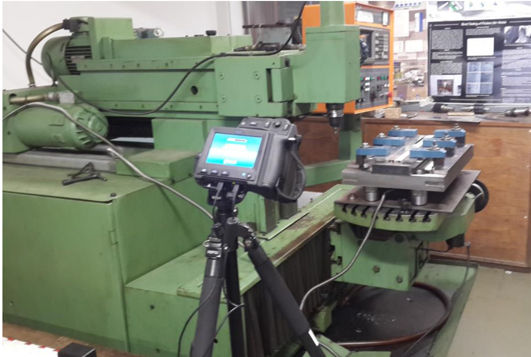
Image 12.11: FLIR thermal camera setup for the during the experiment
