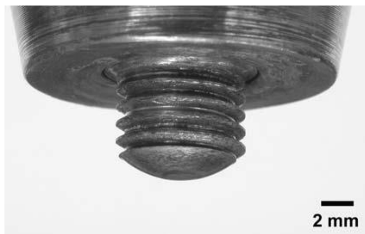
Image 3.3: Photograph of a concave shoulder with a roundbottom pin
