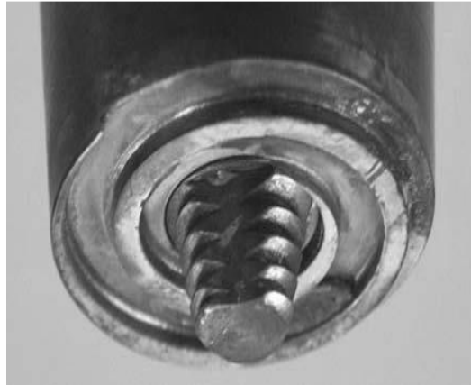
Image 3.1: Photograph of a scrolled shoulder tool and a truncated cone pin containing three flats
