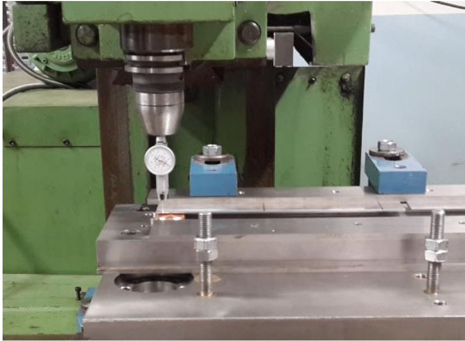
Image 12.3: Finger Gauge Used to set Alignment and Direction of the Tool (Innovative Tool)
