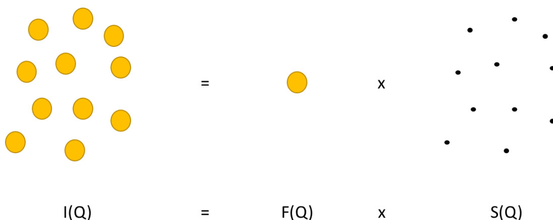
Figure 1.23 The scattering intensity, I(Q) , is a combination of the form factor, F(Q) , and the structure factor, S(Q) .
