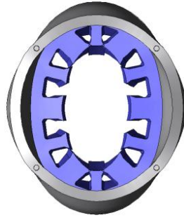
Figure 4.11: Second-order resonant mode shape of 12/10 single-tooth wound segmental rotor SRM
