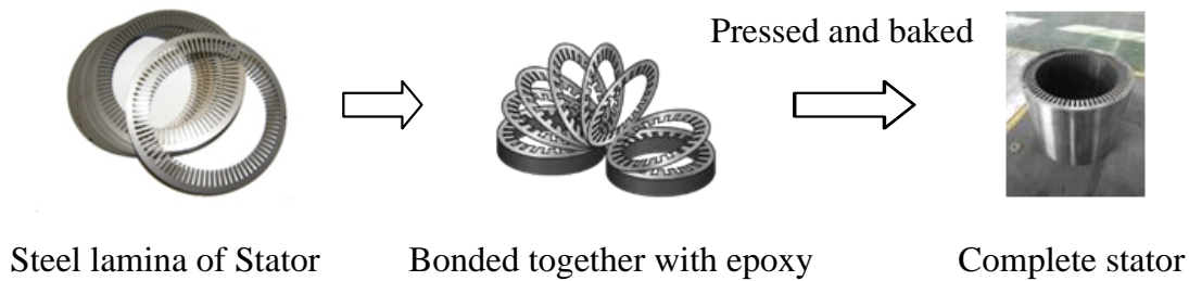
Figure 4.4: Stator lamination core processes
