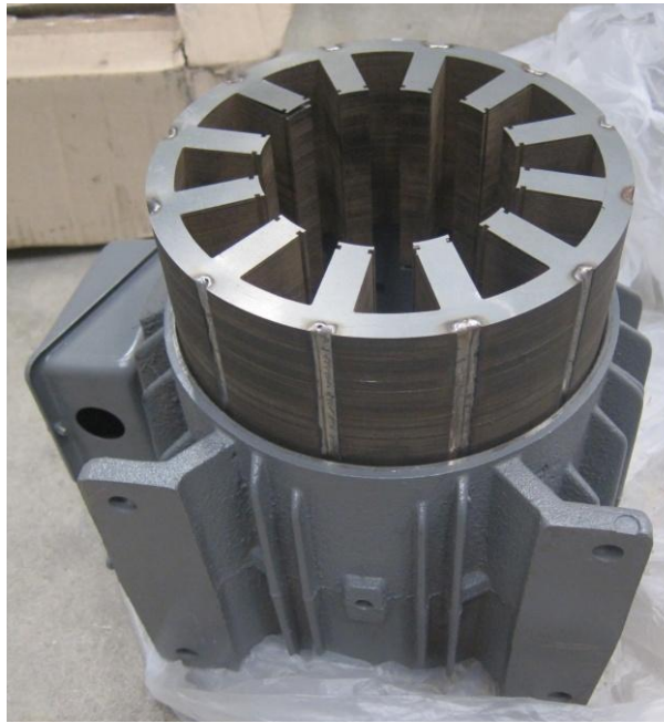
Figure 8.1: Laminated stator core using a welding technique
