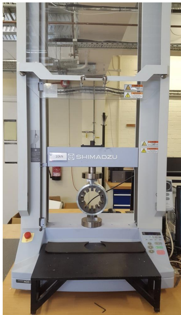
Figure 6.38: The 10 kN Shimadzu Autograph AGS-X material machine testing
