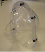
**Figure 3.4. Creating the thermo-plastic shell for the helmet.** (A) Plaster bandages are used to take an impression of the animal's head and a model is created (B). (C) The model is then halved to create a face and back piece (D). Thermal plastic is heated and moulded around the head model using a vacuum forming machine (E). A hand drill is used to cut out areas for the ears, eyes and mouth and to place attachments as needed (F).
