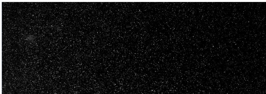
(c) Tracer particle only image, produced by subtracting dilated inertial particles from original combined image.
