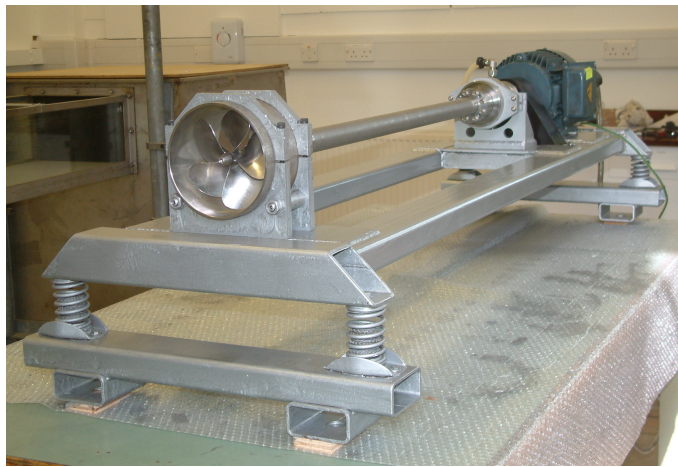
FIGURE 3.2: New axial flow propeller pump, drive shaft tube, seal and motor on vibration isolation cradle.
