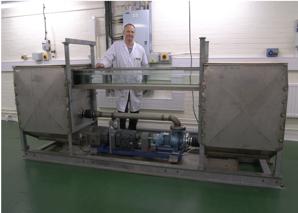
FIGURE 3.1: The original water-channel, as supplied by Dantec and re-assembled at Newcastle.
