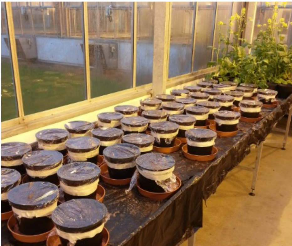
Figure 6.2. Sealed pots after the incorporation of plant material in the first pot trial.
