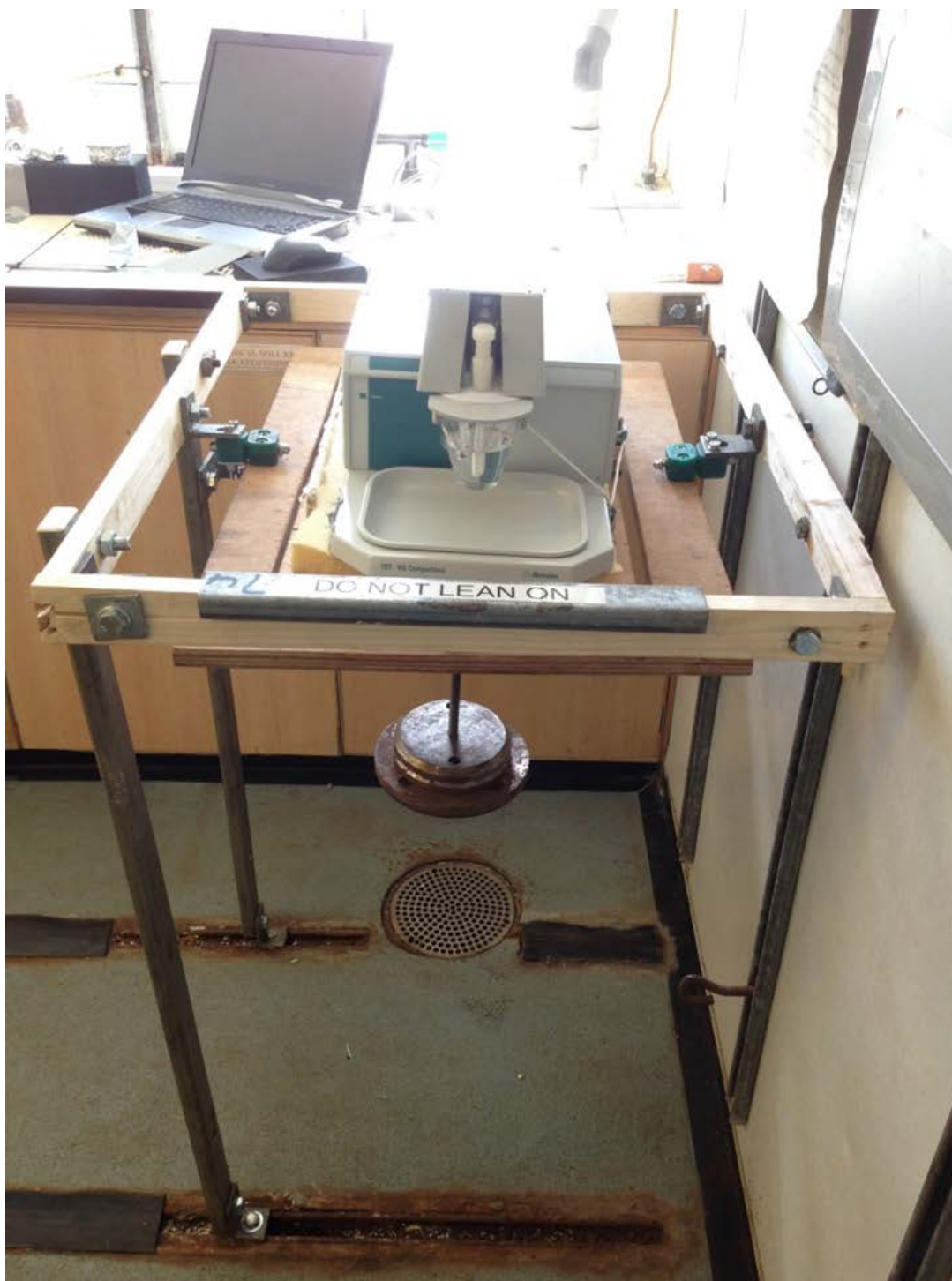
Figure 2.11. 797 VA Computrace on the gimballed table during AMT25 (2015).
