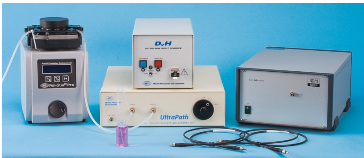
Figure 2.14. (Ultrapath) spectrophotometer with fibre-optic pathlength.
