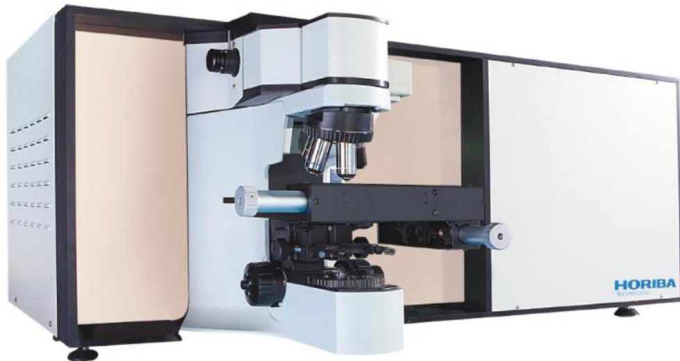
Figure 3-12 LabRAM 800 Raman system used in this work.
