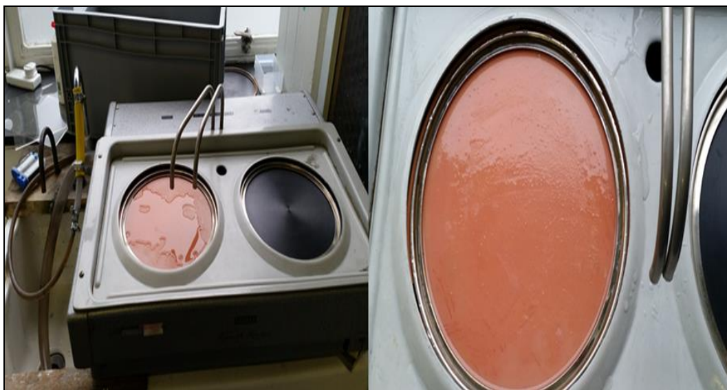
Figure 3-2 Grinding and polishing machine used for preparing the samples.
