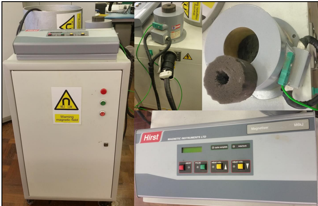
Figure 3-11 Magnetiser and pick-up coil for magnetizing the samples.
